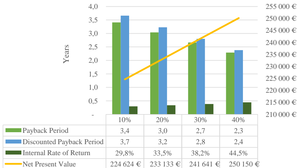
Figure 8. Financial parameters of investment in the PV system according to the changes in funding
